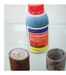
Cleansing of the heat exchanger by antirzhavin, which production technology is developed by researchers of the TSU Laboratory of Catalytic Research, entered the list of the best practices of Rosneft. The product is recommended to be used by all oil-refining plants of the company.
